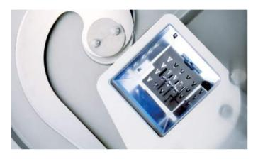
Thanks to a perfect grip on the product, parallel slices and highest yields are possible even for bone-in products. A look in the blade box shows a thin blade for a precise cut.
