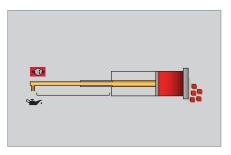
The **hygiene cylinder** (supplied as standard) makes product contamination with hydraulic oil a technical impossibility. No oil can enter the cutting chamber. **Double seals** on the gridset shafts and the blade shaft seal the machine interior even better against the ingress of foreign bodies and moisture.
