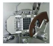
FlexRotationSystem technology makes it possible to adjust the blade speed ideally to the specific product and application (100 to max. 400 rpm). It simply couldn't be more flexible.
