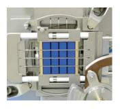
TWISTER SP+ premium cube: The cutting chamber is initially fully closed for optimum product compression. The product is measured and cut leaving no trim.
