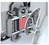
Excellent cutting results thanks to the patented gentle cut gridset (optional). This ensures the best possible cutting geometry for excellent cutting results, without tempering the products, particularly with delicate products such as cooked meat or boiled sausage.
