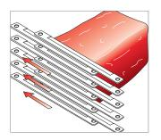
The unique dual-stroke, twopart grid system facilitates precise dicing and stripe dicing of the most delicate products by providing twice the nor-mal cutting length at reduced cutting pressure.
