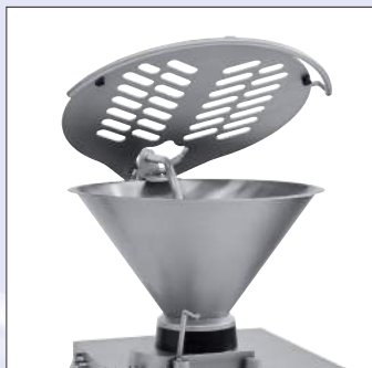
casing holding device, fixed for natural casings
