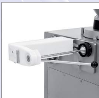
casing holding device, fixed for natural casings
